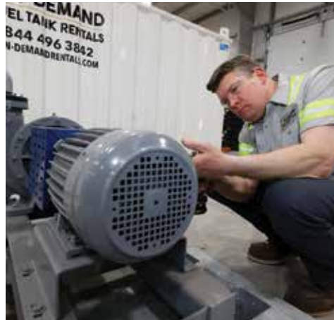
Jason Neilson, a fuel technician, services an external fuel pump inside the company's shop.
